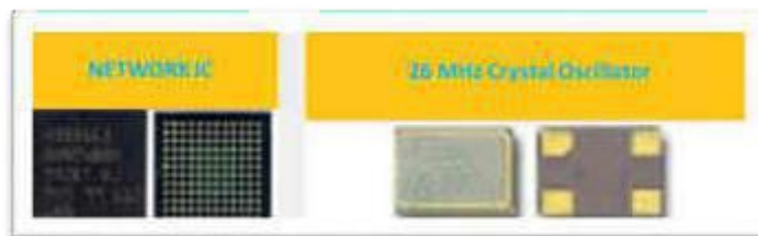
Fig. 2.2.4(ii): Network IC and 26 MHz crystal oscillator of a mobile
