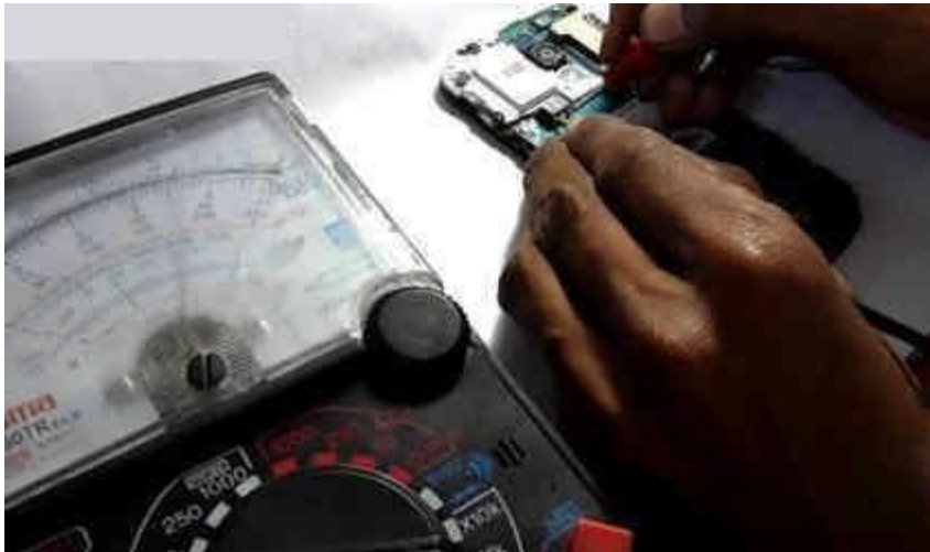
Fig. 2.5.6.3: Checking shorting with multimeter
