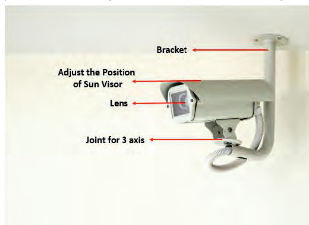
Fig 5.3.2: CCTV placed on a ceiling
