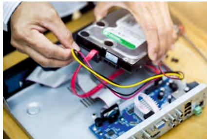
Fig 5.1.1(c): Placing hard disk within DVR
